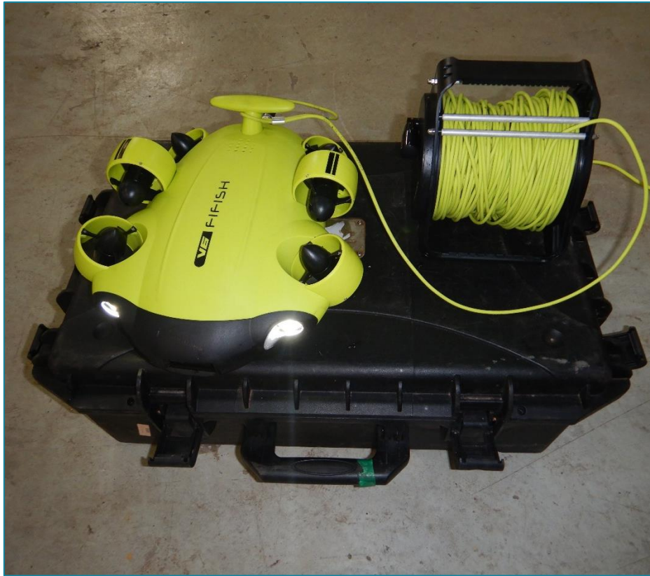
Figure 5: QYSEA Fifish HD ROV
