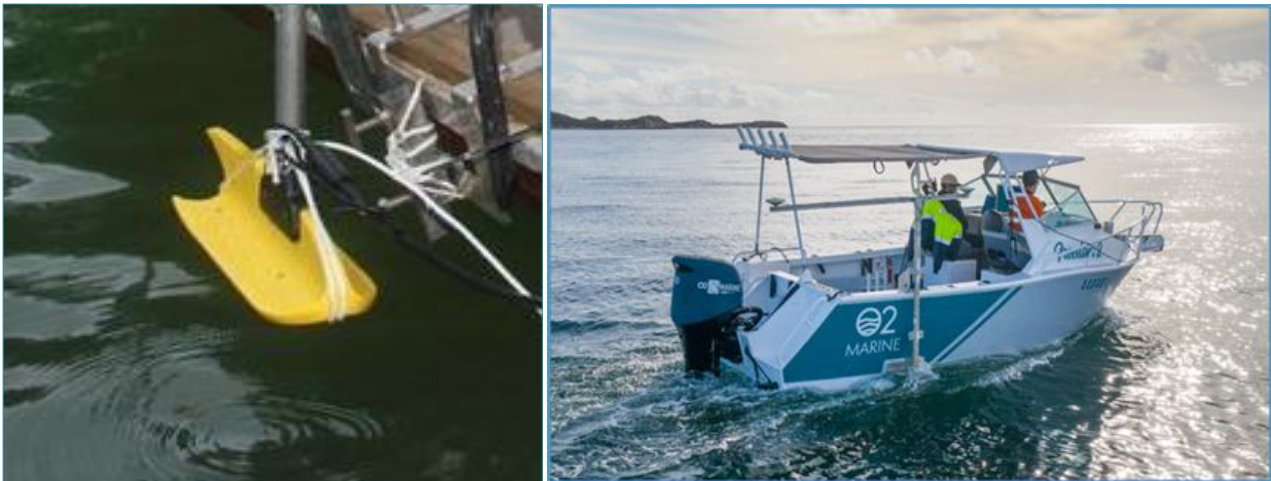
Figure 4: Example pole mounted Starfish Sidescan Sonar, Freedom II vessel undertaking survey.
