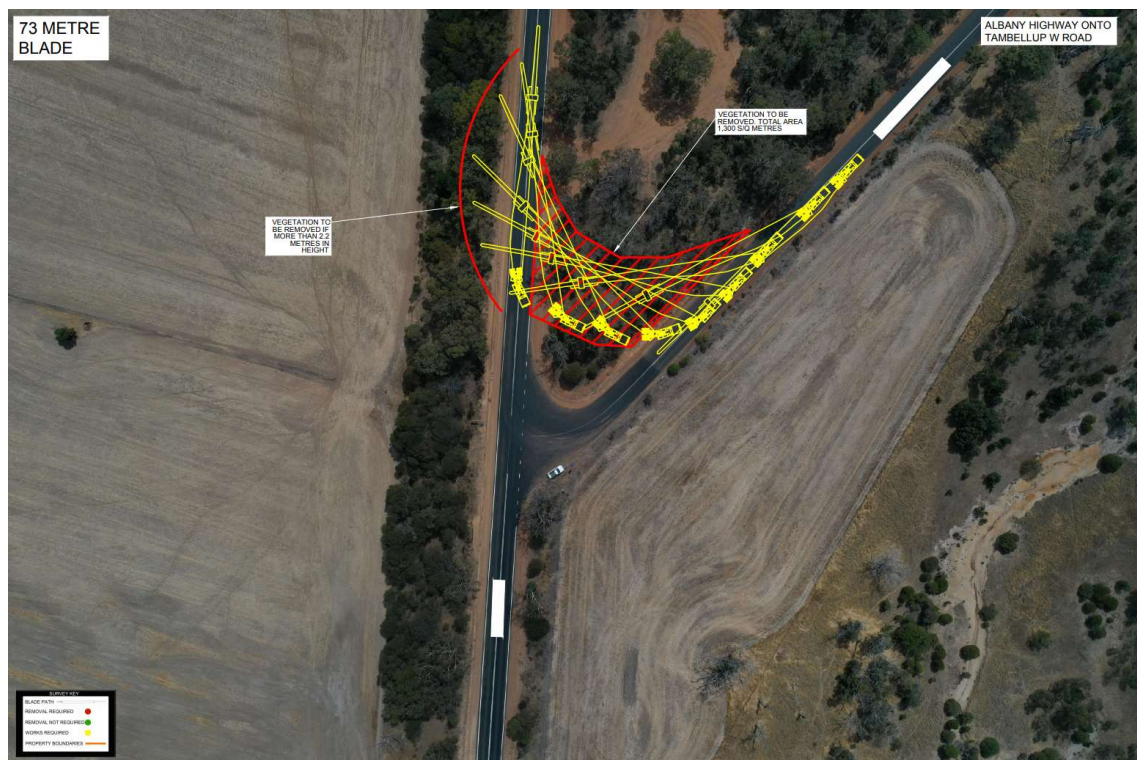
Figure 4: Tambellup Road trailer Sweep path analysis. Existing trees marked area where clearing will need to be taken (red).
