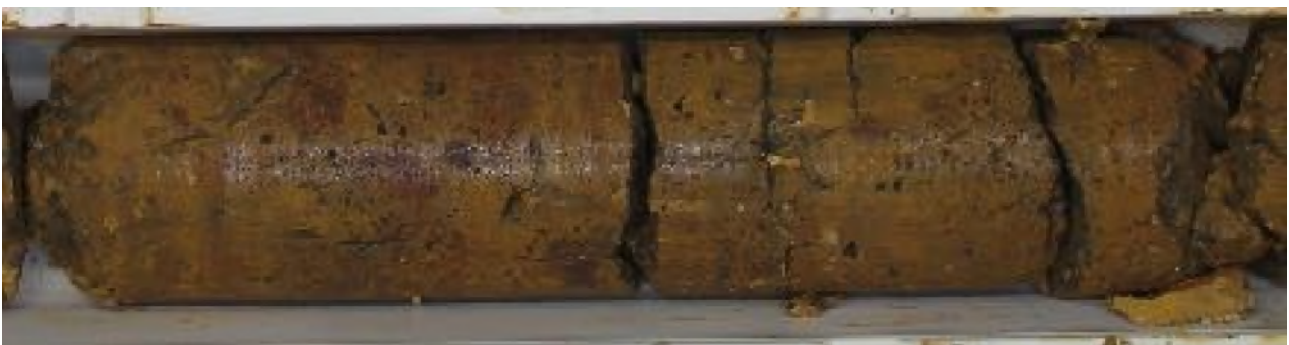
Figure 3.30: Diamond core of CID-upper layer depicting vugs and fractures (CZR 2023)
