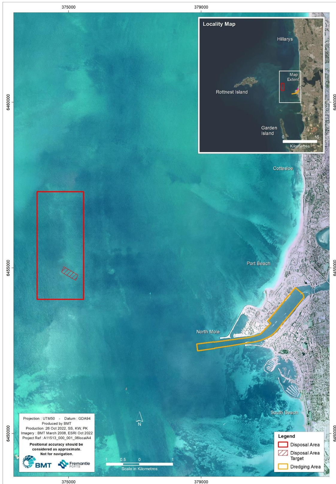
Figure 1.1 Dredging plan within the Inner Harbour (yellow polygon) and disposal plan west of Gage Roads (red rectangular).
