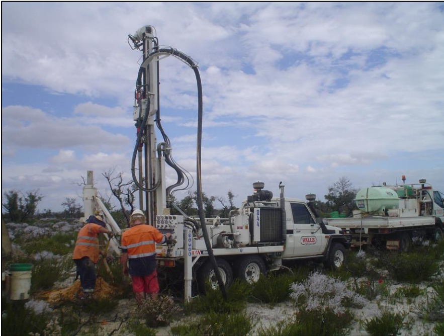
Plate 2 Example of exploration drill rig which avoid large scale clearing by driving over and around vegetation instead of removal
