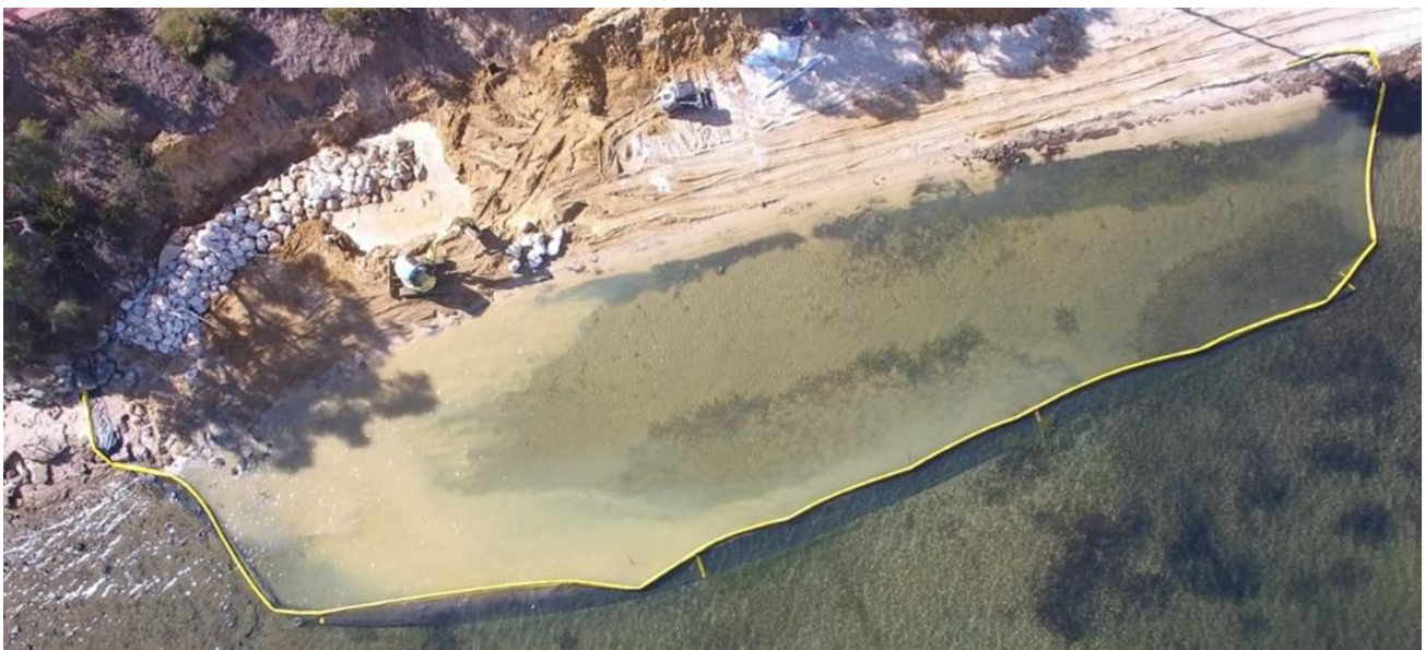
Figure 2: Natural Area silt curtain deployed at Point Heathcote Reserve, Applecross (2016).
