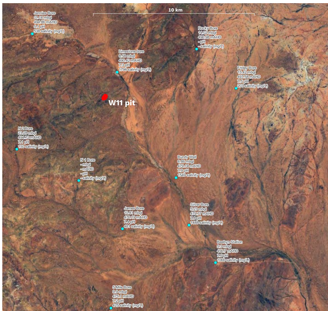
Figure 8 Bores close to W11 - including results of a bore audit in 2008 (data from SRK, 2008)
