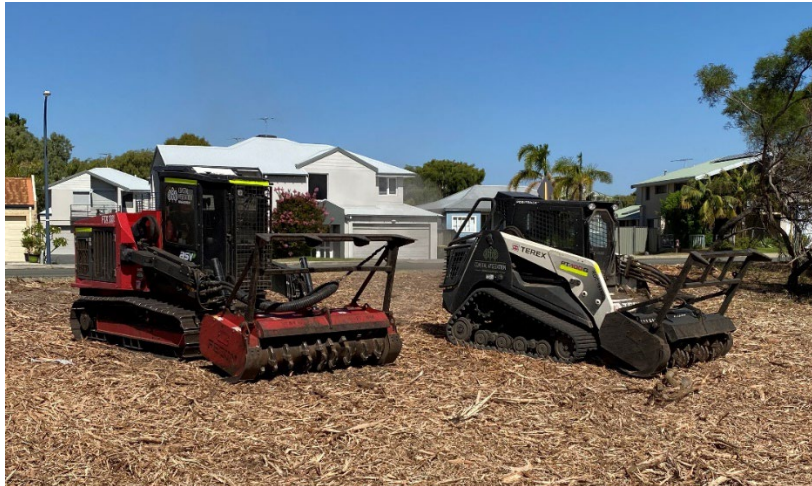
Image 3: Falcon Forestry Mulching Machine – 2200mm wide & Terex Positrack with Fecon Forestry Mulcher Attachment – 1900mm wide
