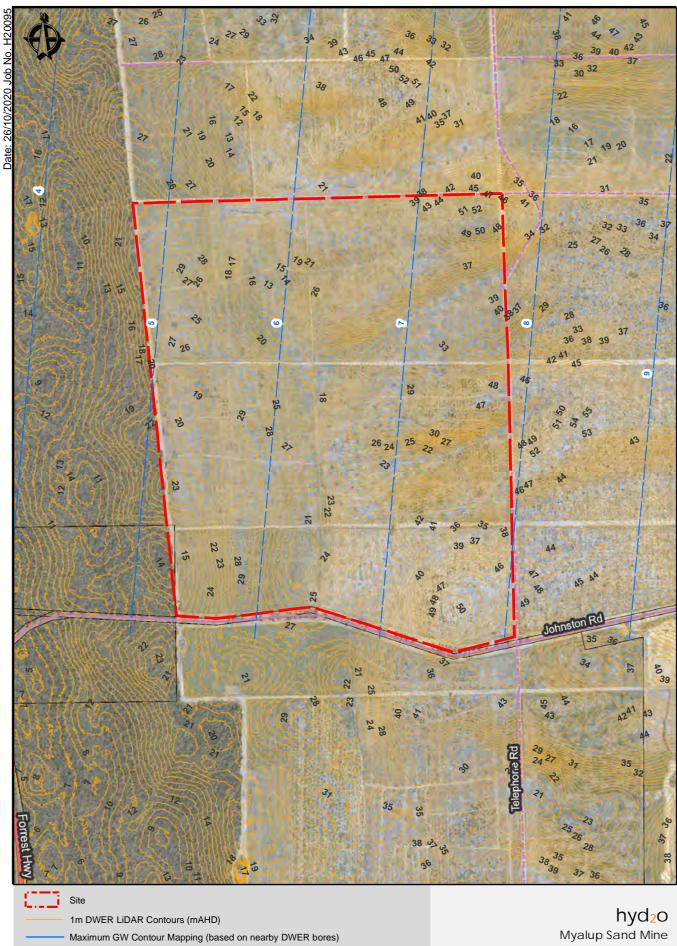
Maximum GW Contour Mapping (based on nearby DWER bores) Site Groundwater Map & LiDAR
