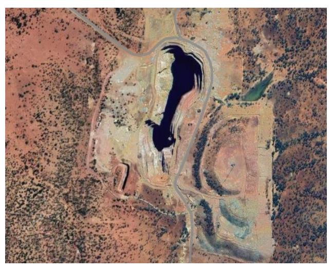
Figure 5: Flooding Caused by Past Damming of Ephemeral Drainage at Reichelt's Find
