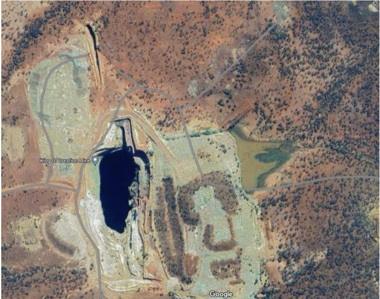
**Figure 4: Flooding Caused by Past Damming of Ephemeral Drainage at King of Creation**
