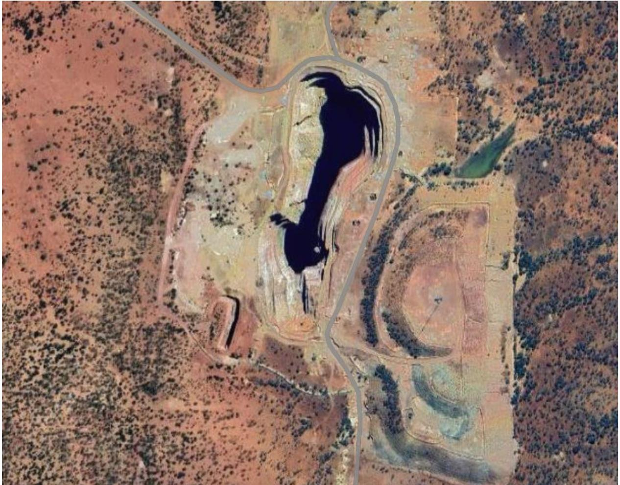
**Figure 5: Flooding Caused by Past Damming of Ephemeral Drainage at Reichelt's Find**
