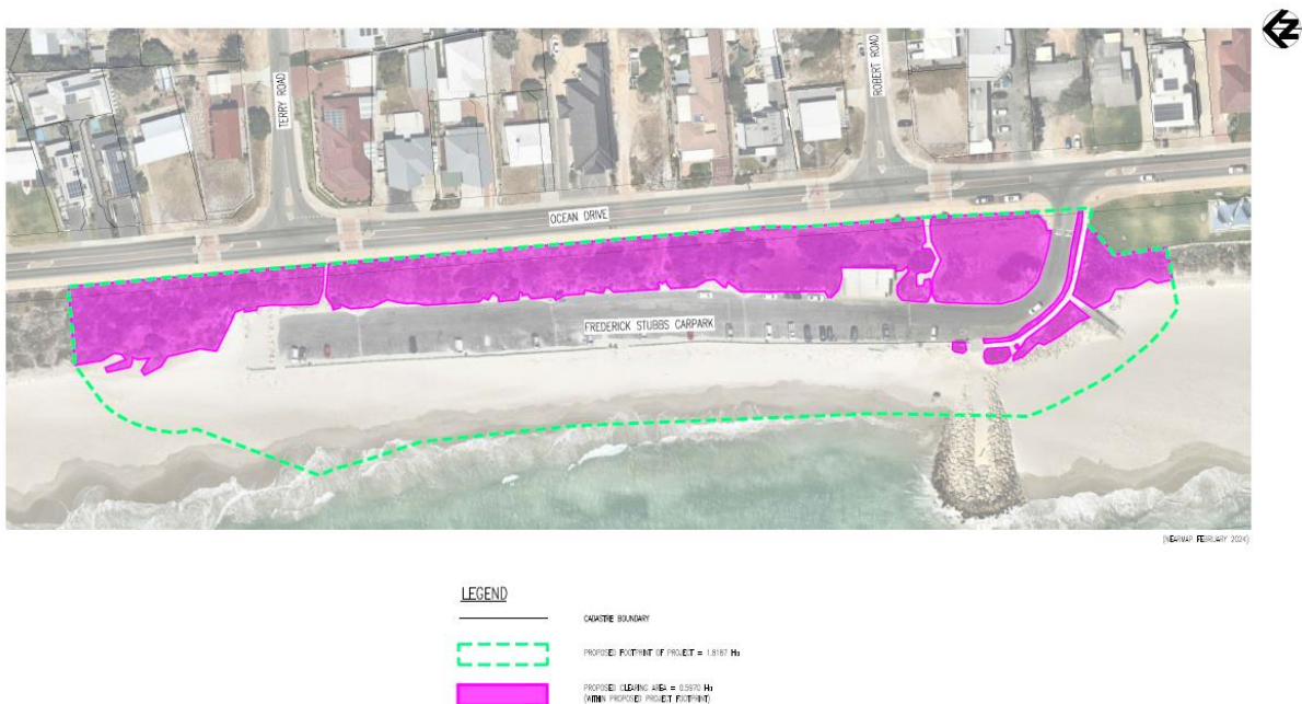
Figure 4 Location of the proposed Frederick Stubbs Carpark clearing area, totaling 0.597 hectares (5,970m 2 ) to support the upgrades to the existing carpark infrastructure, QUINNS ROCKS.
