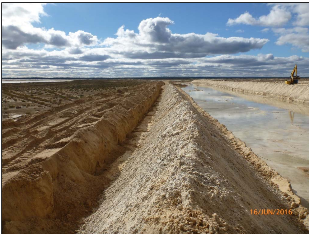
Plate 16: Strip mining sequence showing of quarry excavation (RHS), gypsum windrow (middle) and topsoil material as outer windrow (LHS)
