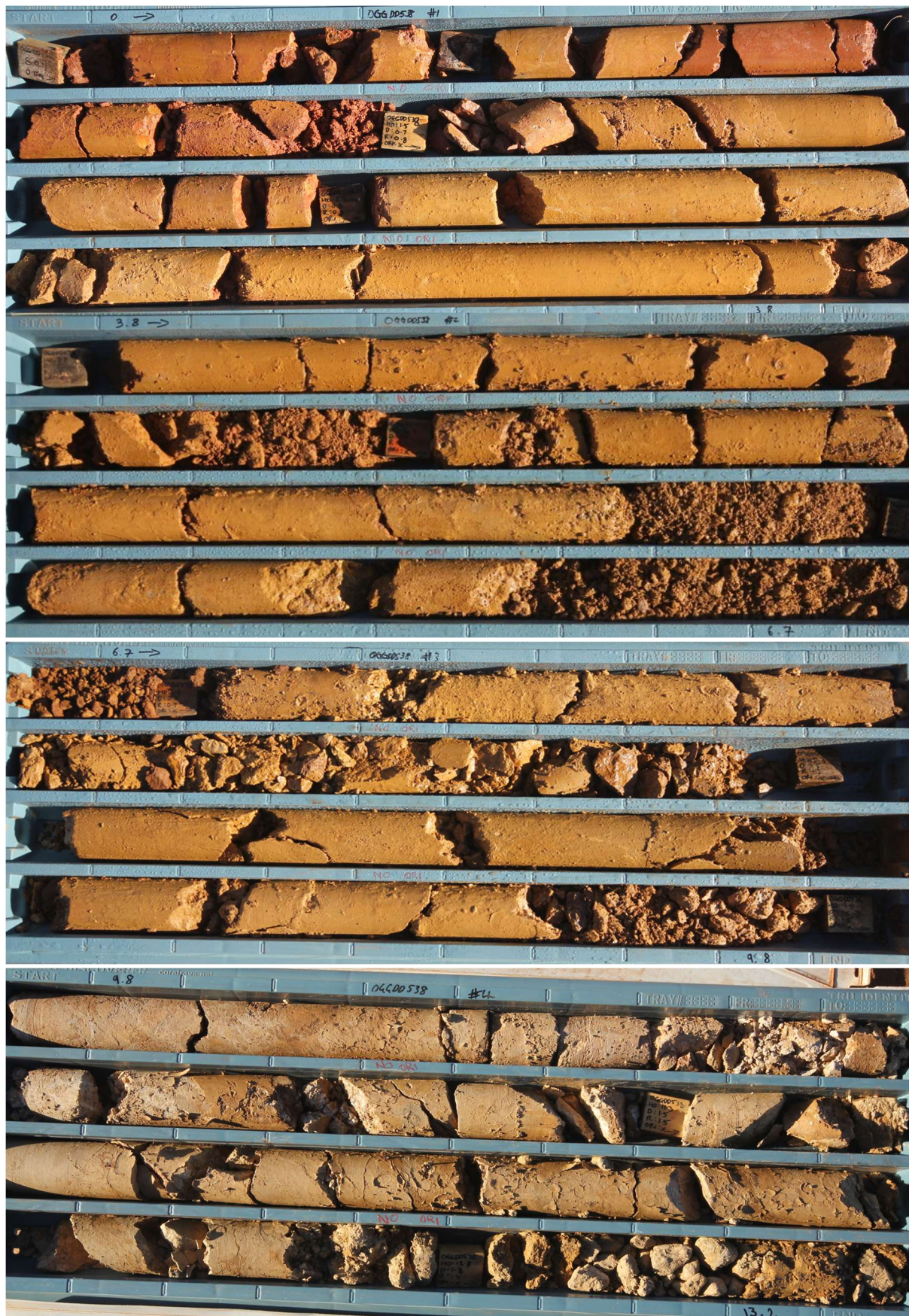
Plate 4: Unsaturated geological sequence at site OGGDD538 (0 to 13.2 m below ground level), located in the south-western part of the deposit.
