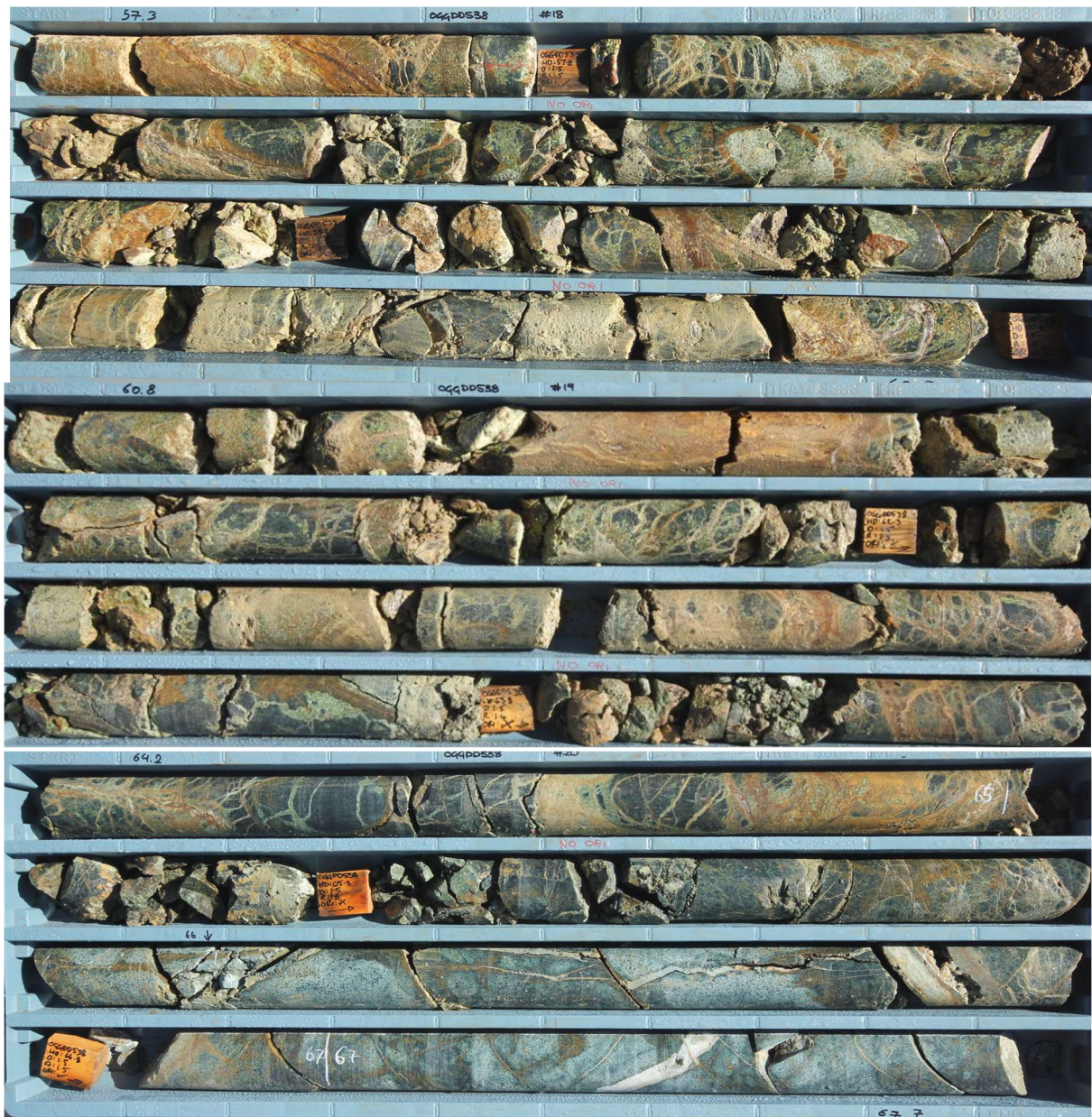
Plate 8: Saturated geological sequence at site OGGDD538 (57.3 to 67.7 m below ground level), located in the south-western part of the deposit.
