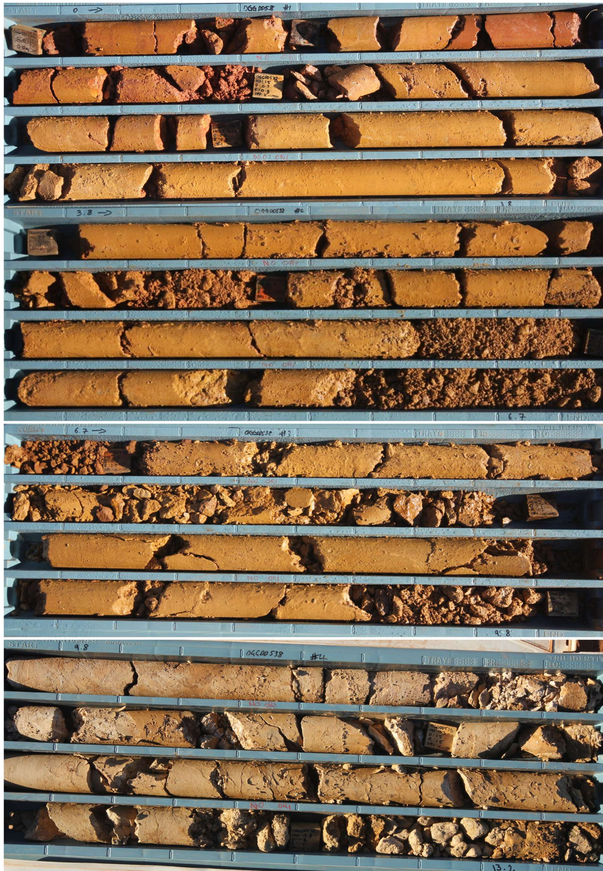
Plate 4: Unsaturated geological sequence at site OGD538 (0 to 13.2 m below ground level), located in the south-western part of the deposit.
