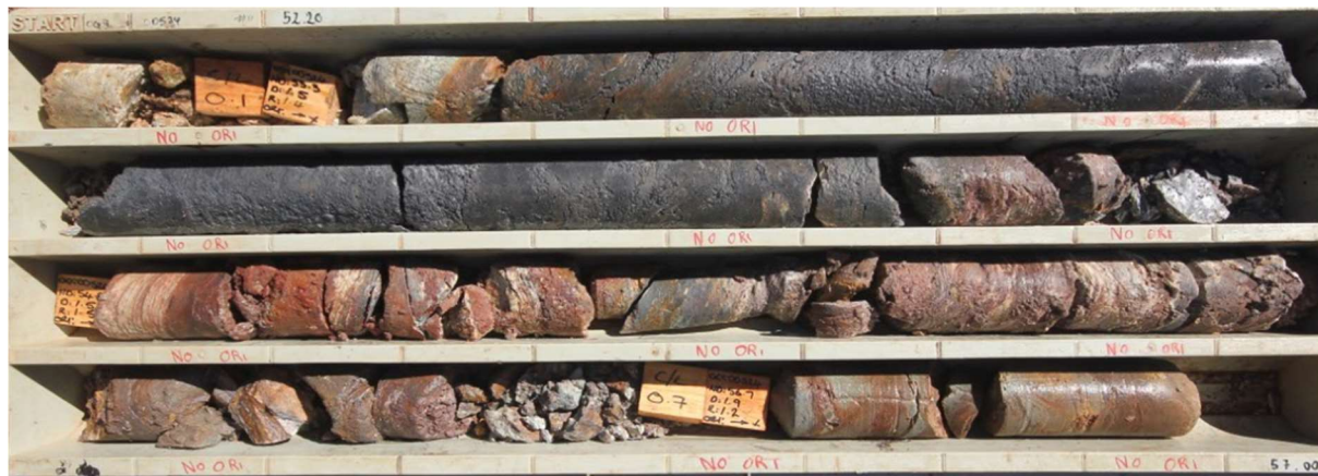
Plate 5: Saturated geological sequence at site OGGDD524 (52.2 to 57 m below ground level), located in the central part of the deposit.
