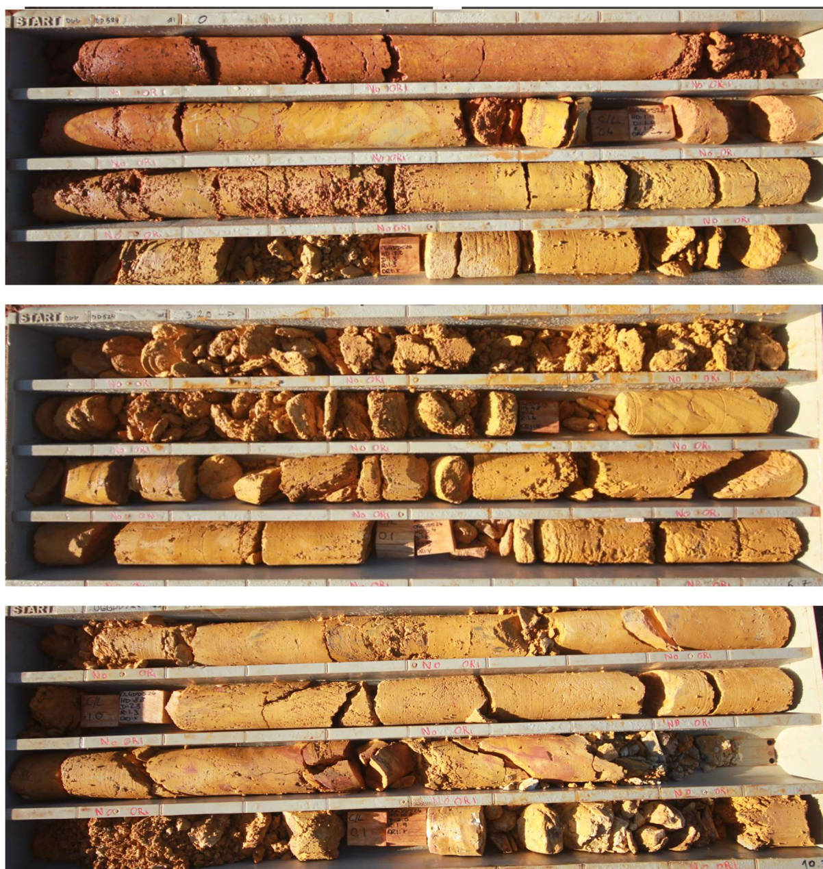
Plate 1: Unsaturated geological sequence at site OGGDD524 (0 to 10.3 m below ground level), located in the central part of the deposit.
