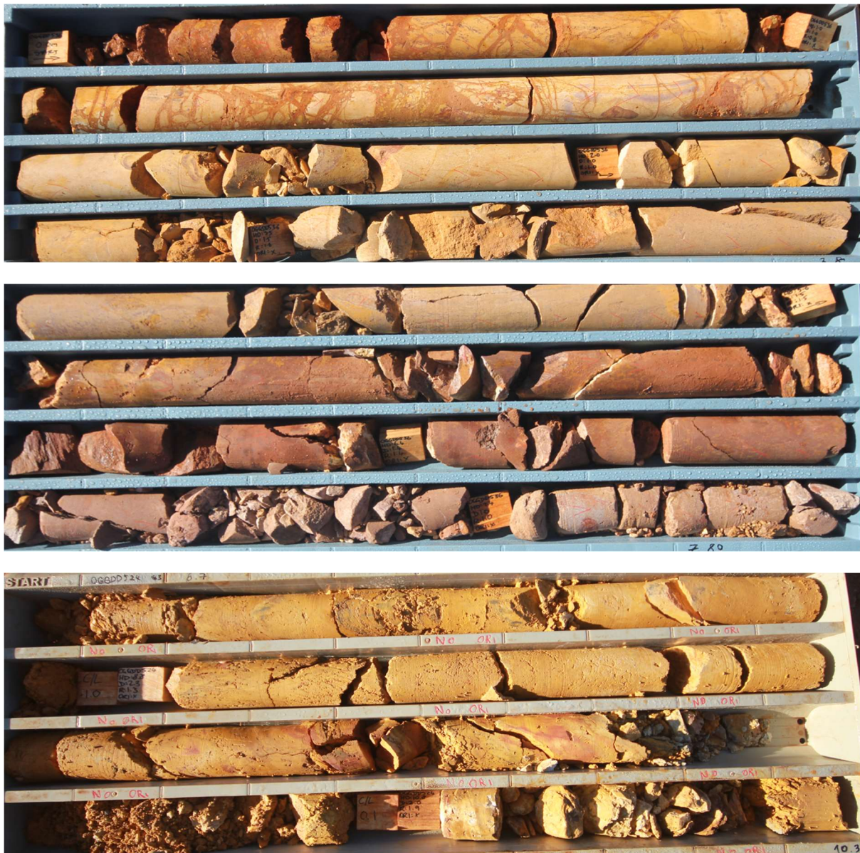
Plate 2: Unsaturated geological sequence at site OGGDD536 (0 to 10.3 m below ground level), located in the central part of the deposit.
