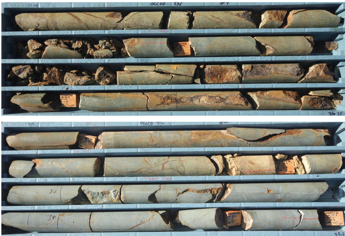
Plate 6: Representative core photograph at site OGGDD536 (31 to 38.7 m below ground level), located in the central part of the deposit.
