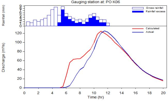
Graph 3: Tuflow (actual) vs RORB (calculated) hydrograph; 2% AEP 12-hour
