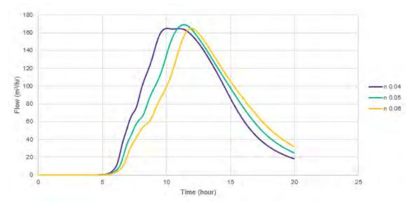
Graph 4: Comparison of Catchment Outlet Hydrograph for Various Roughness
