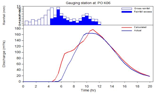
Graph 2: Tuflow (actual) vs RORB (calculated) hydrograph; 1% AEP 12-hour
