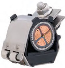
DESCRIPTION: SINGLE CABLE CLEAT (CABUS 5864 OR (ELLIS) MANUFACTURER: IPD PART NUMBER: EPVRT-03 FINISH: 316L STAINLESS STEEL WITH INTEGRATED LSF HALOGEN POLYMERIC LINER & BASE PAD.
