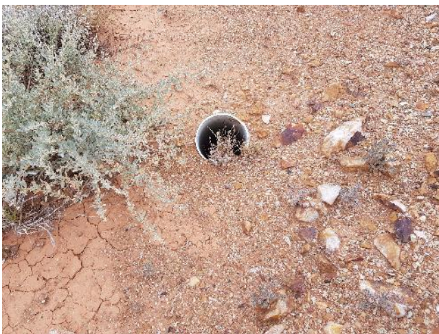
Plate 21. Uncapped exploration drill hole
