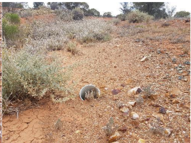
Plate 22. Uncapped exploration drill hole
