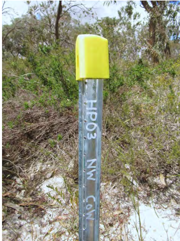
Plate 1 Quadrat marking method. 90cm steel droppers with yellow safety caps. NW and SE corners.
