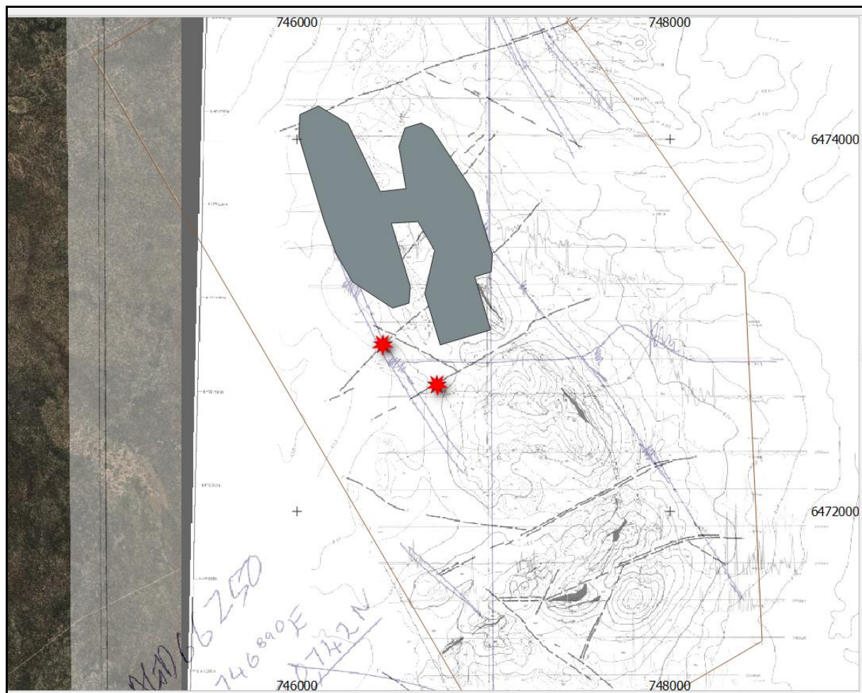
Figure 1: GDA94 MGA Z50 translated from AGD using QGIS. Red stars show position of interpreted shear for drilling.
