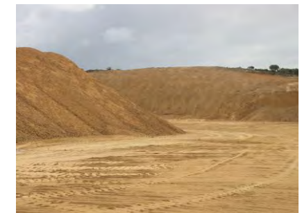
Typical operational pit with walls providing visual and noise screening and stockpiles on the floor of the pit
