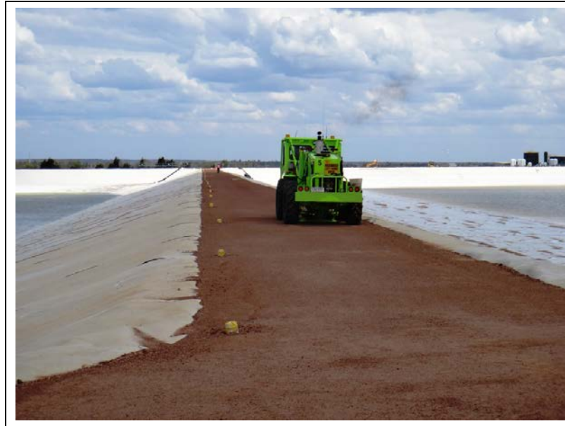
Plate 3.4. Vibroseis vehicle working in an active group of nodes
