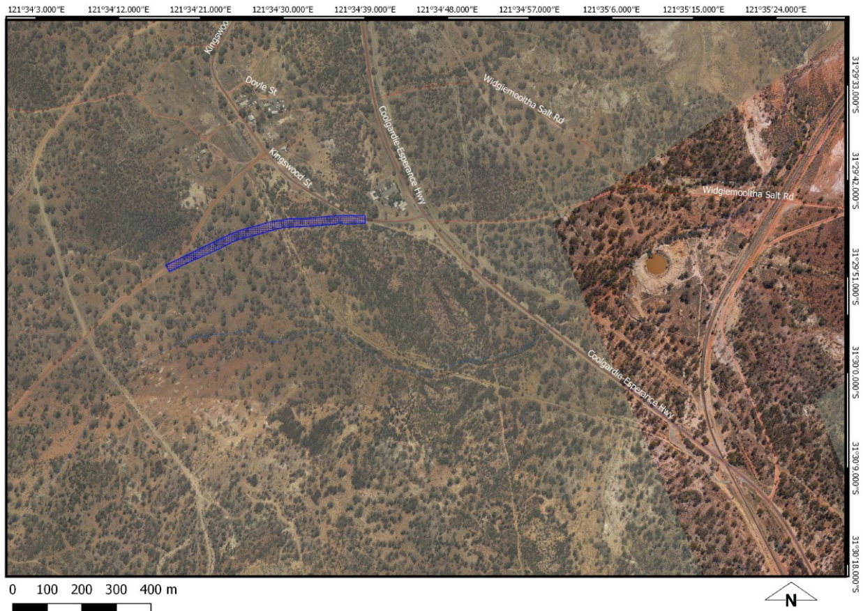
Figure 2: The clearing area (shown in blue), shown in comparison to the existing road centrelines (depicted in red). Defined surface water features are also shown (depicted by the blue lines).
