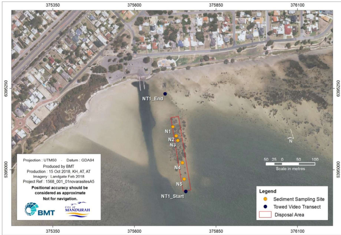
Figure 2.1 Survey sites and towed-video transect at Novara boat ramp disposal area, October 2018
