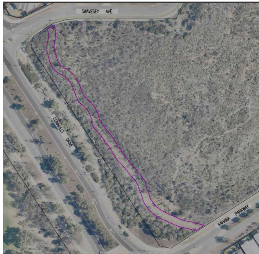
Figure 3: Proposed clearing of 1,165m 2 for the construction of a fire access track on the western side of Kahana Park, Butler (City of Wanneroo 2021b).
