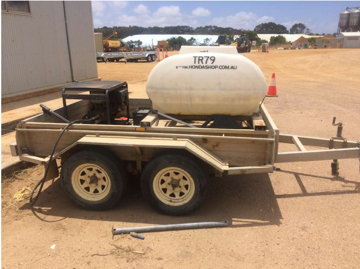
Figure 2: One of the Shire of Esperance's fleet of mobile washdown facilities
