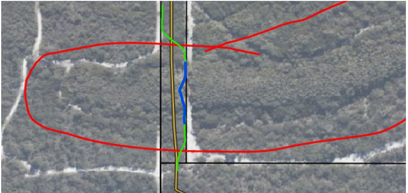
Figure 4 – Proposed trail alignment in seasonally inundated wetland area (approximate extent circled in red) in northern portion of alignment. The yellow line represent the originally proposed trail alignment, the blue line indicates a portion of the revised trail alignment where the boardwalk is planned to be constructed to minimise impacts to the wetland, and the green line indicates a portion of the revised trail alignment where a trail is planned to be constructed along the ground surface.
