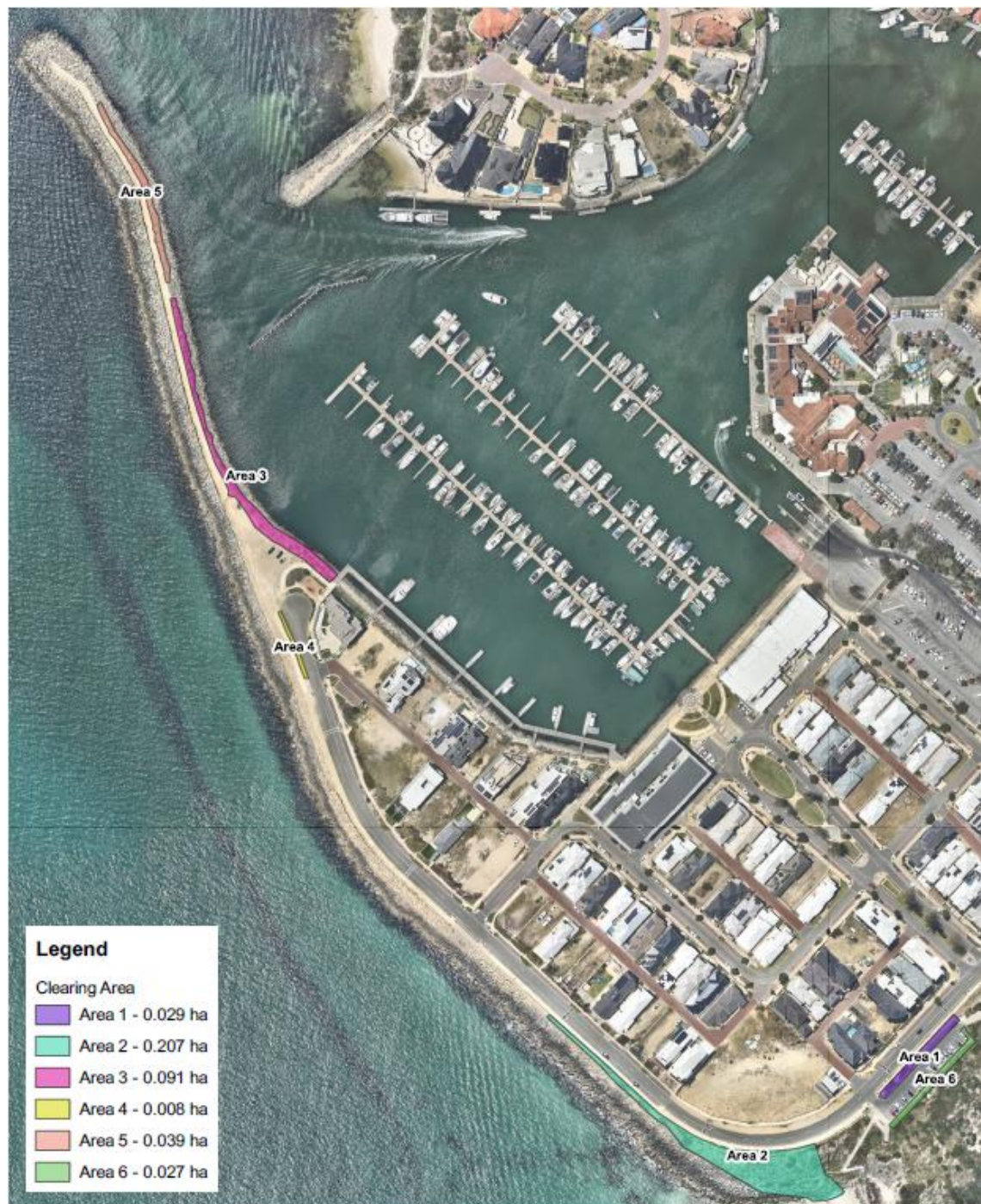
Figure 2: Proposed clearing of 0.401 hectares for the renewal of the Mindarie Breakwater, upgrades to the Clayton's Beach carpark and upgrades to drainage along Alexandria View, Mindarie. The segmented upgrade works for the Mindarie Breakwater include Clearing Areas 2, 3, 4 and 5. Upgrades to the carpark include Clearing Areas 1 and 6.
