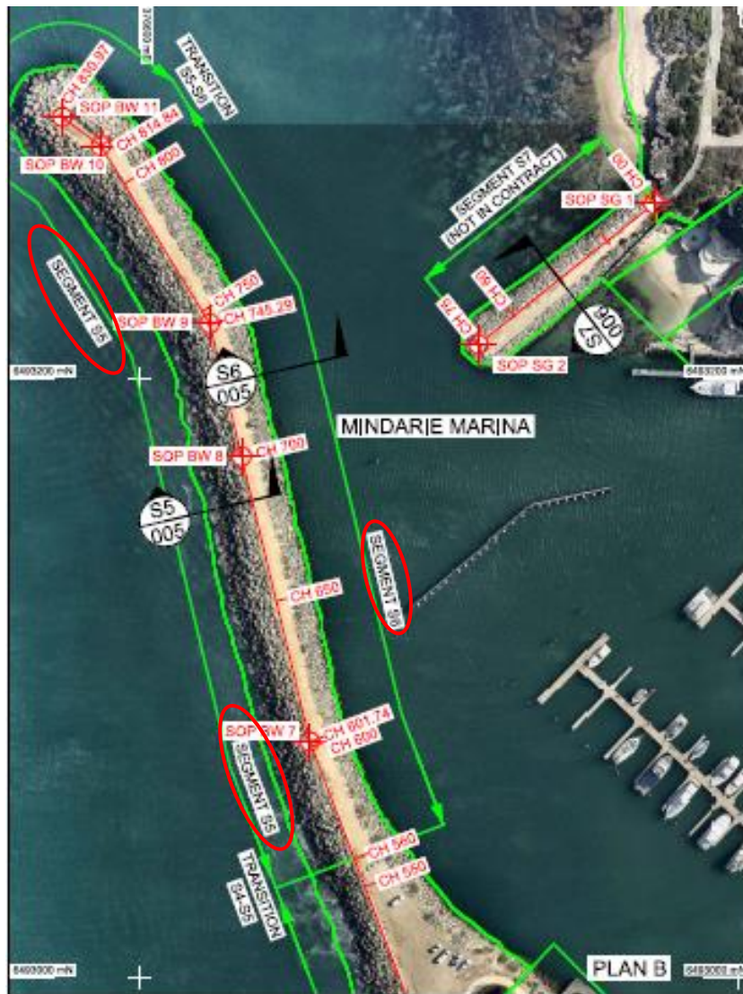
Figure 3b: Design plan detailing locations of segments (circled in red).
