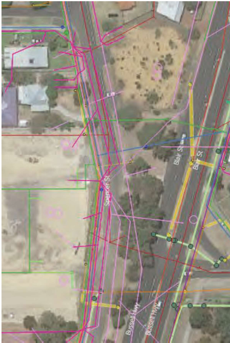
Figure 31: Screenshot from GIS model showing DBYD data of Spencer St near Bussell Hwy/Blair St
