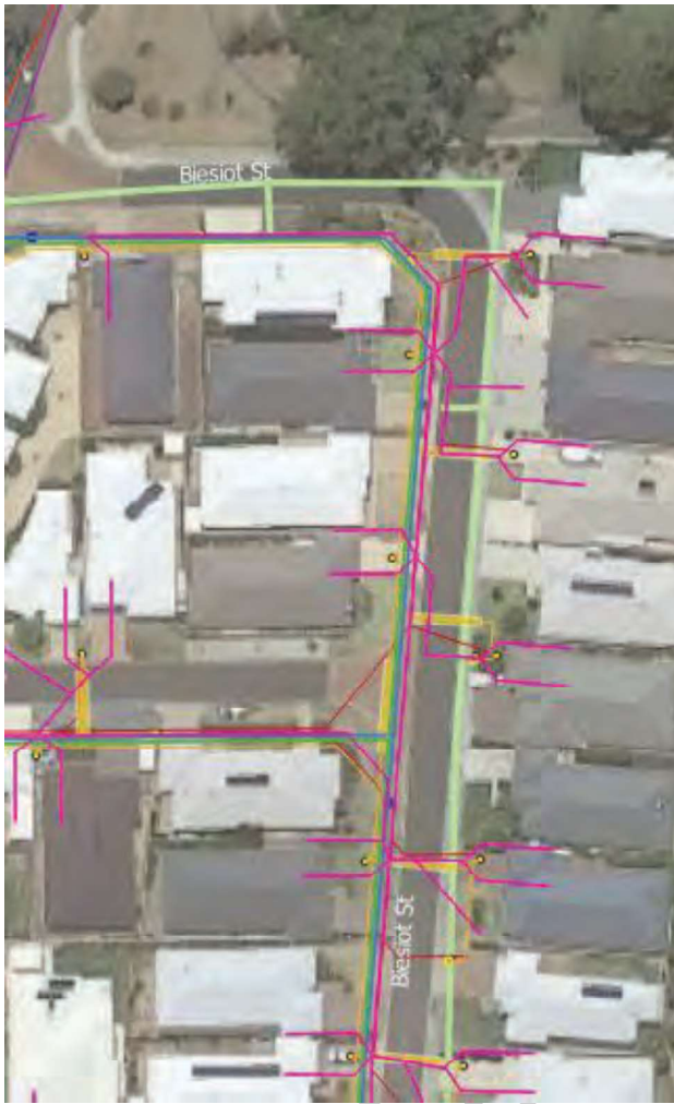
Figure 36: Screenshot from GIS model showing DBYD data for Biesiot St north of Gorman Loop
