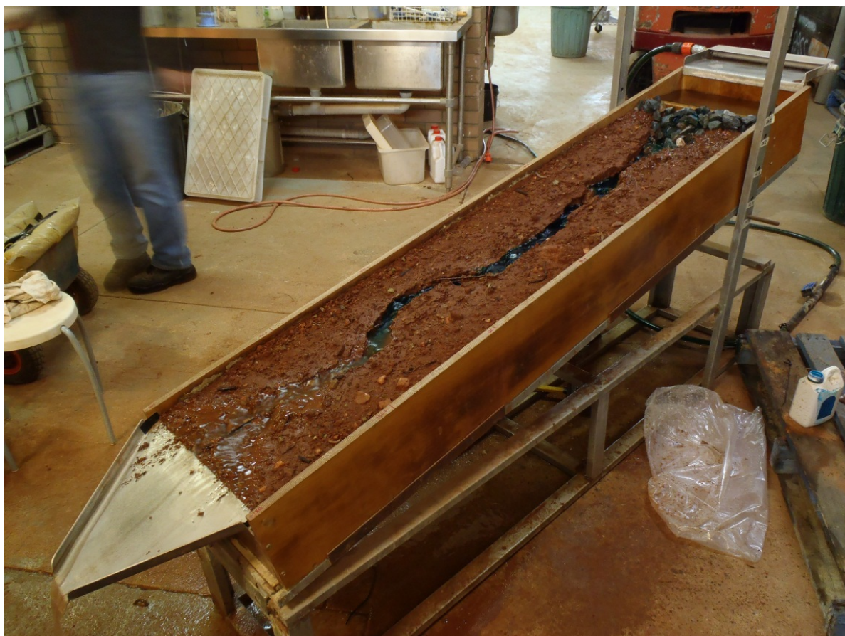
Plate 3.3: Laboratory-scale rill erosion test.
