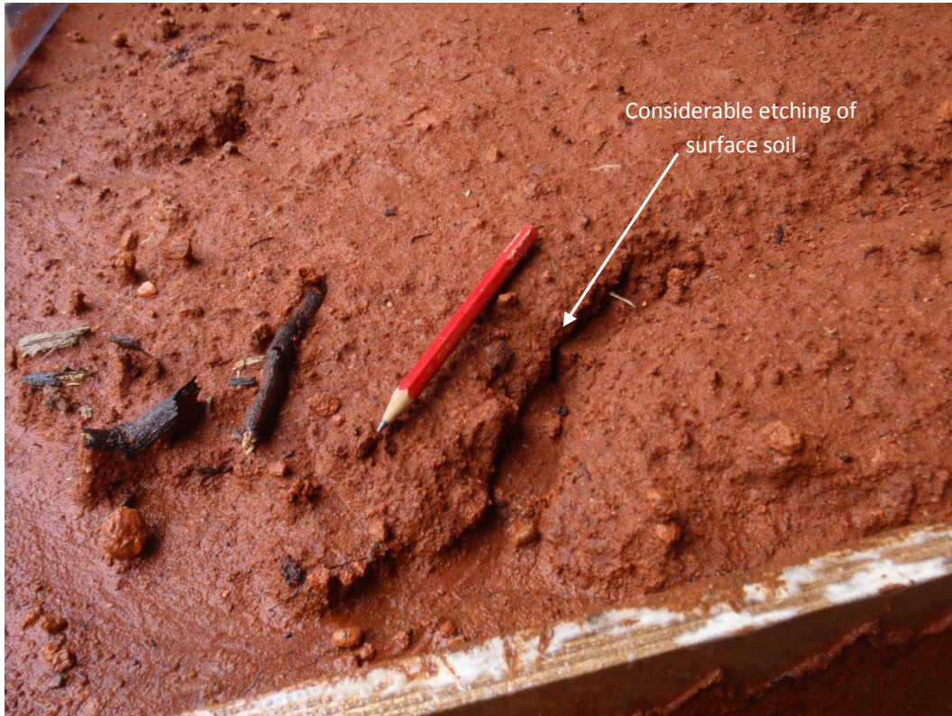
Plate 4.16: Response of the Hornet surface to applied rainfall at a slope angle of 15°.
