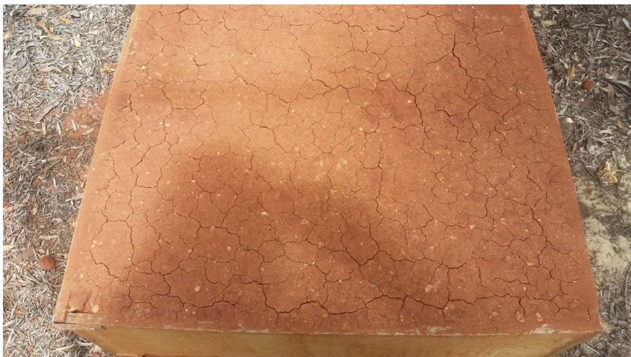
Plate 3.2: Laboratory rainfall simulator after wetting/drying cycle
