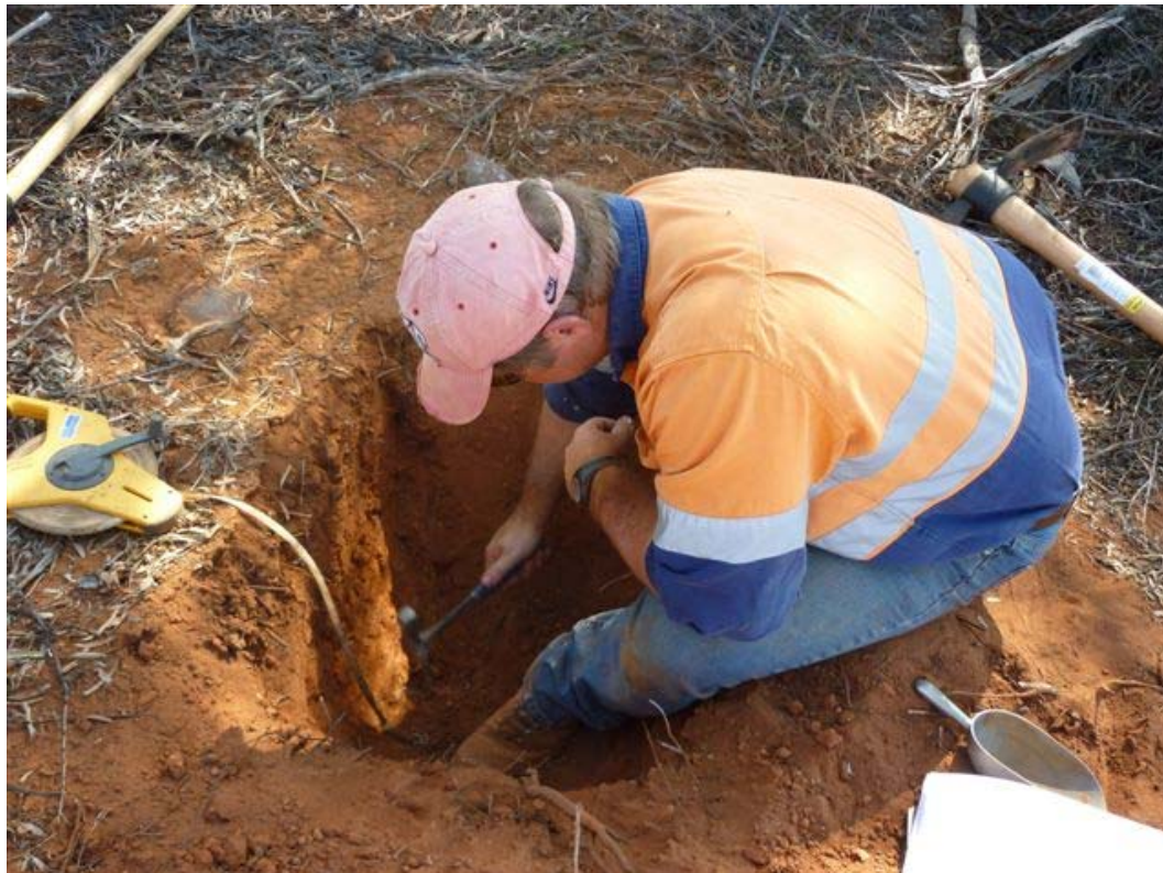
Plate 3.1: Excavation of shallow soil trenches by hand to characterise the surface soils.
