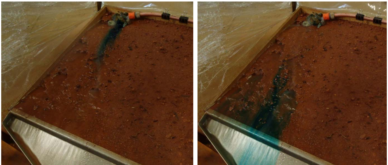
Plate 3.4: Laboratory-scale “mini-flume” rill erosion test.
