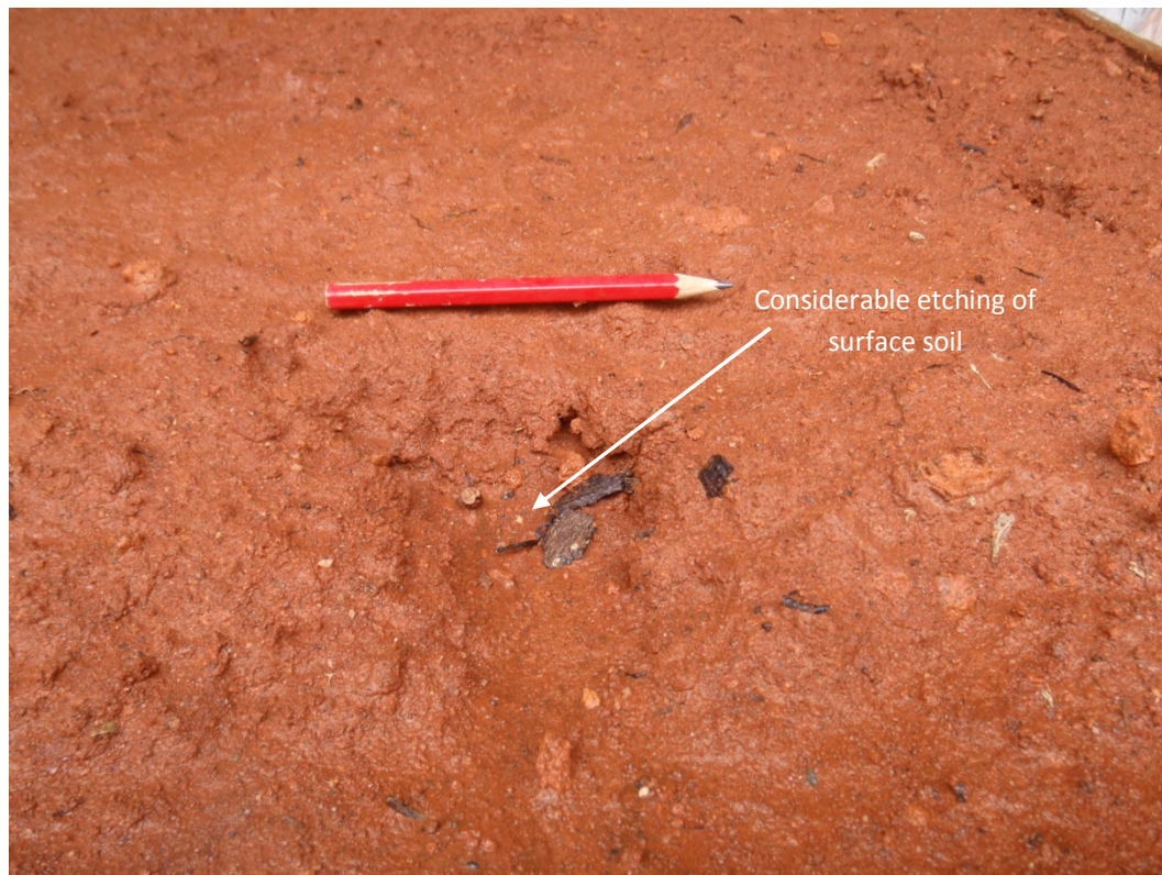
Plate 4.15: Response of the Hornet surface to applied rainfall at a slope angle of 12°.
