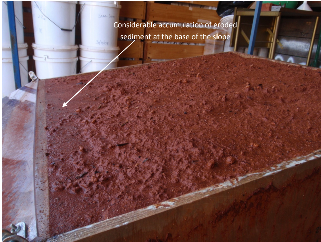
Plate 4.14: Response of the Hornet surface to applied rainfall at a slope angle of 10°.
