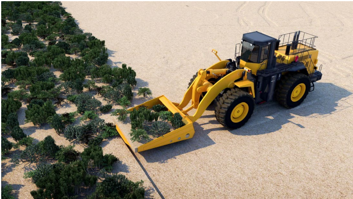
Figure 5: VDT Excavation (sod removal method)
