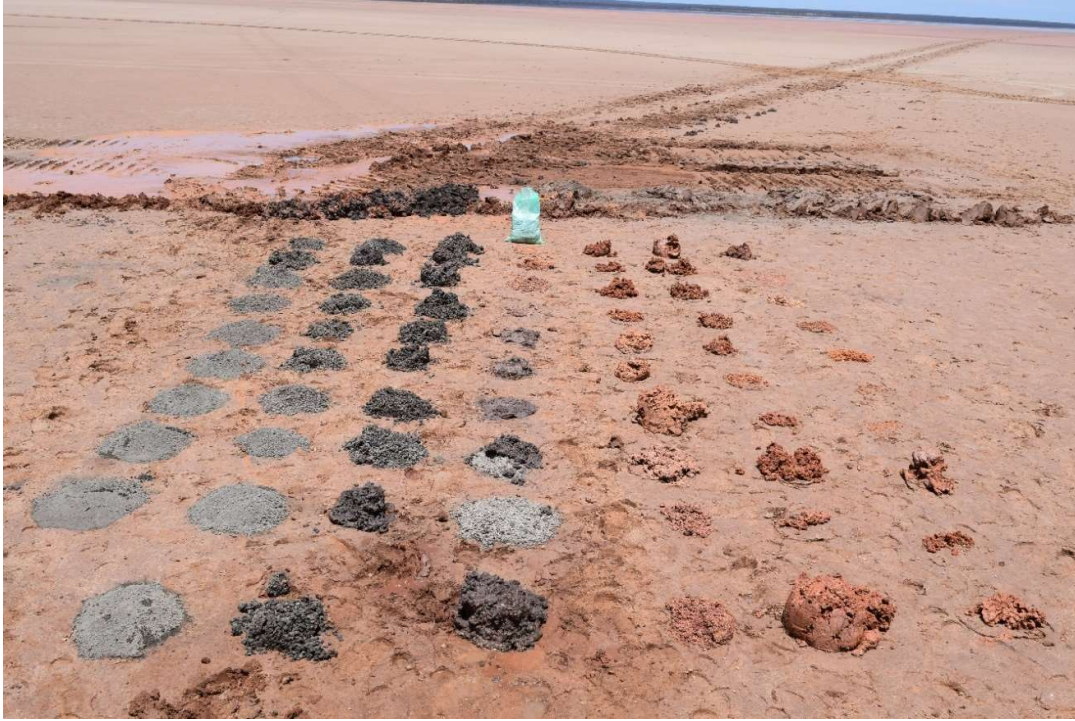
Figure 12: Example of aircore sample piles on the drill pad surface (on-lake drilling)
