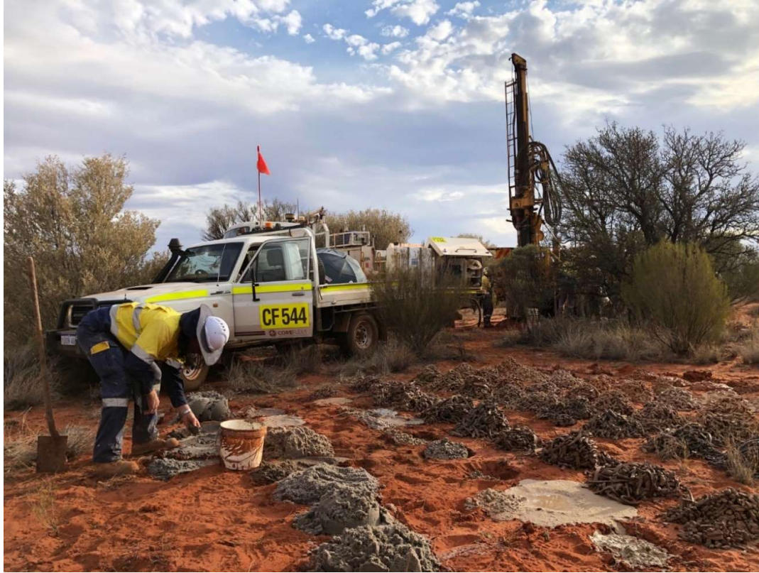
Figure 11: Example of aircore sample piles on the drill pad surface (off lake drilling)
