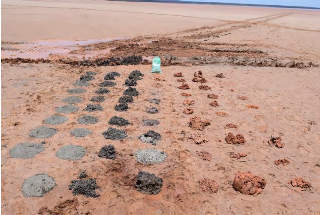
Figure 13: Example of aircore sample piles on the drill pad surface (on-lake drilling)
