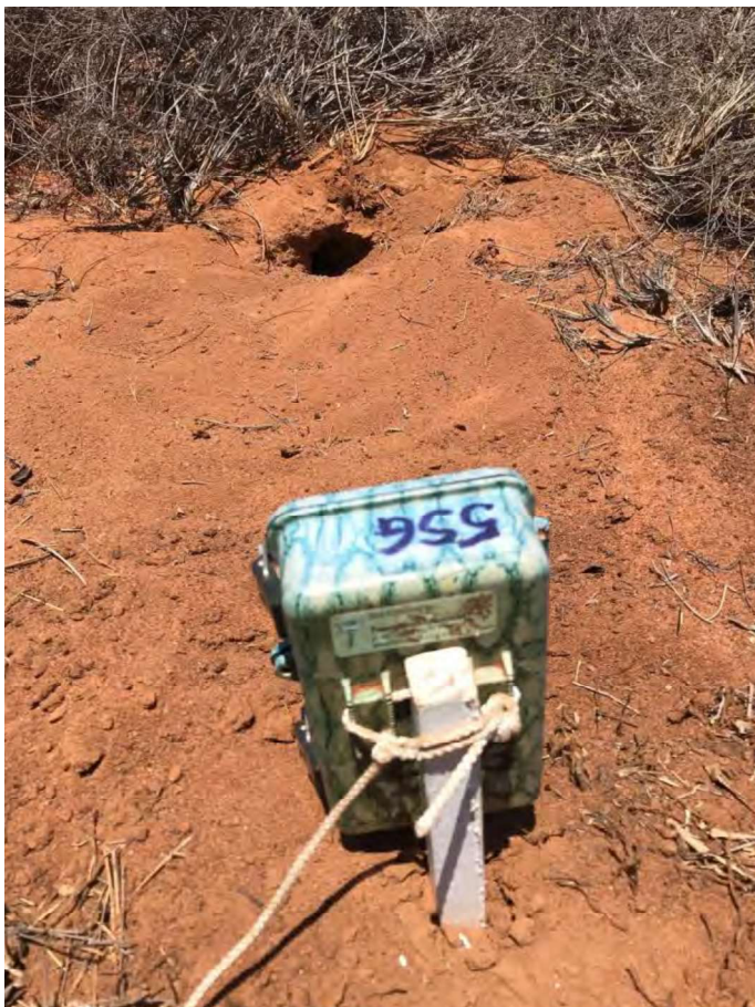
Figure 1 Camera installation method at Mulgara burrows
