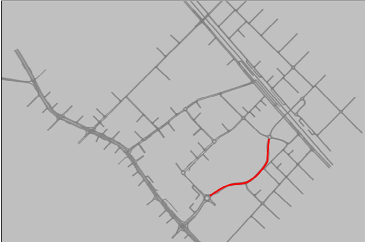
Figure 5-2 Canning City Centre VISSIM Micro-Simulation Model Network and Extents - with Southern Link Road
