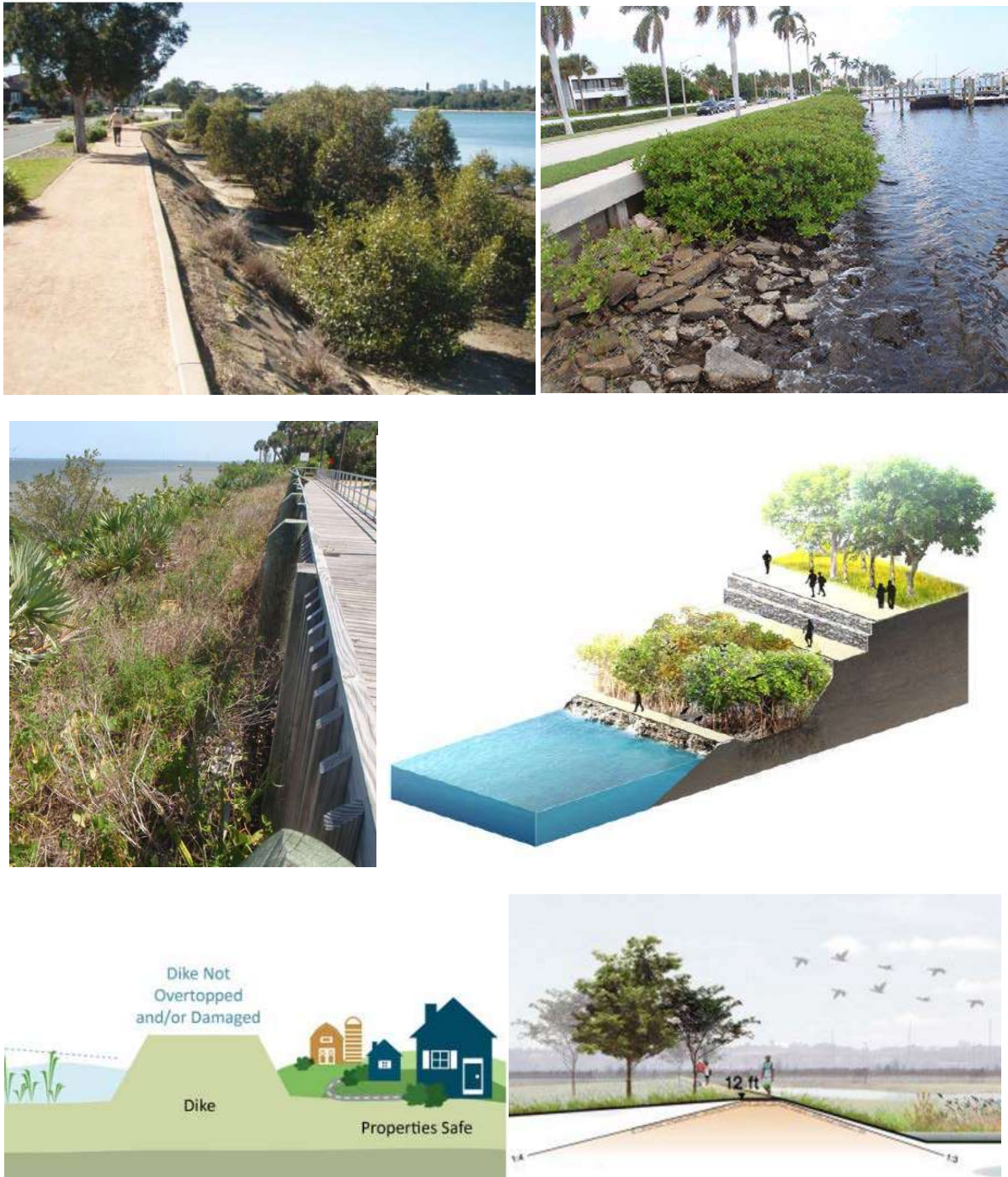
Figure 6.17: Adaptation examples. Sloping seawall (upper left), Vertical seawall with mangrove planter at base (upper right), feature walkways (middle), levy / dike structures (lower)
