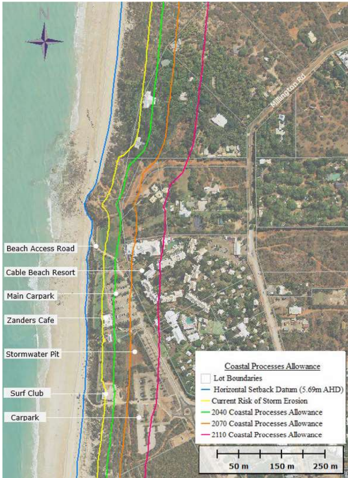
Figure 4.2: Cable Beach Coastal Compartment (Central) showing coastal processes erosion allowances recommended for future planning periods
