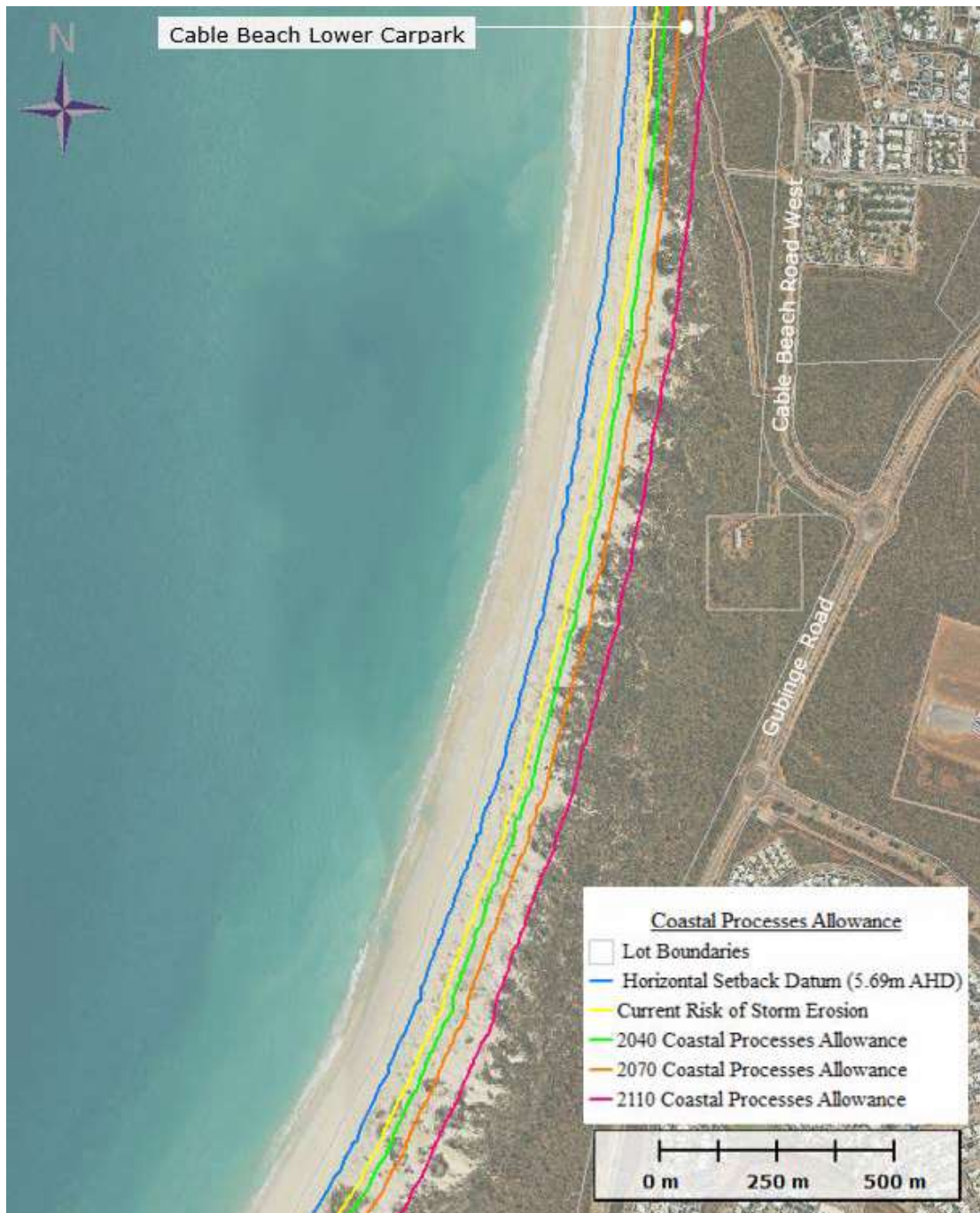
Figure 4.4: Cable Beach Coastal Compartment (South, upper) showing coastal processes erosion allowances recommended for future planning periods
