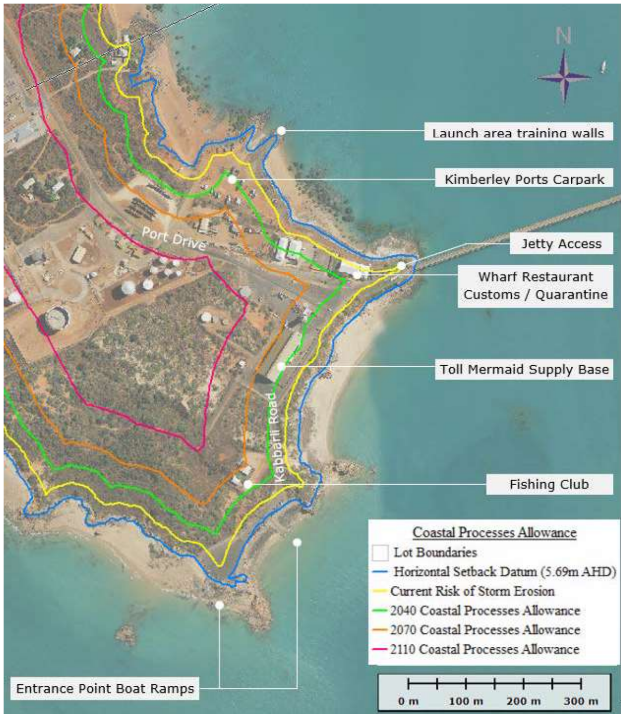
Figure 4.9: Entrance Point Compartment (east side) showing coastal processes erosion allowances recommended for future planning periods
