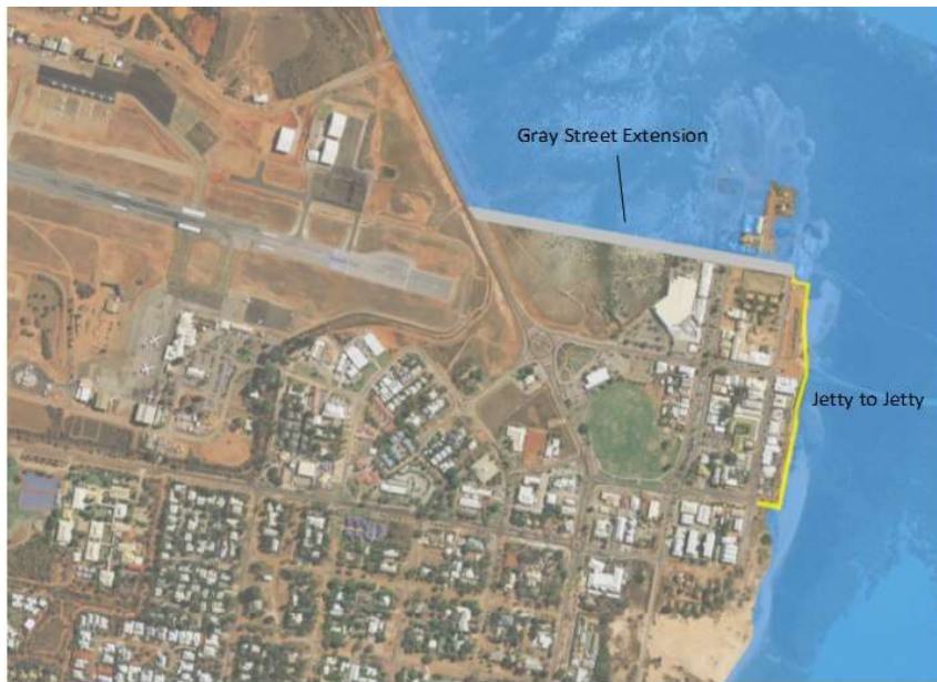
Figure 6.23: Concept Option 2 proposing Gray Street Extension as coastal protection structure across northern side and seawall/walkway on eastern side of Chinatown.
