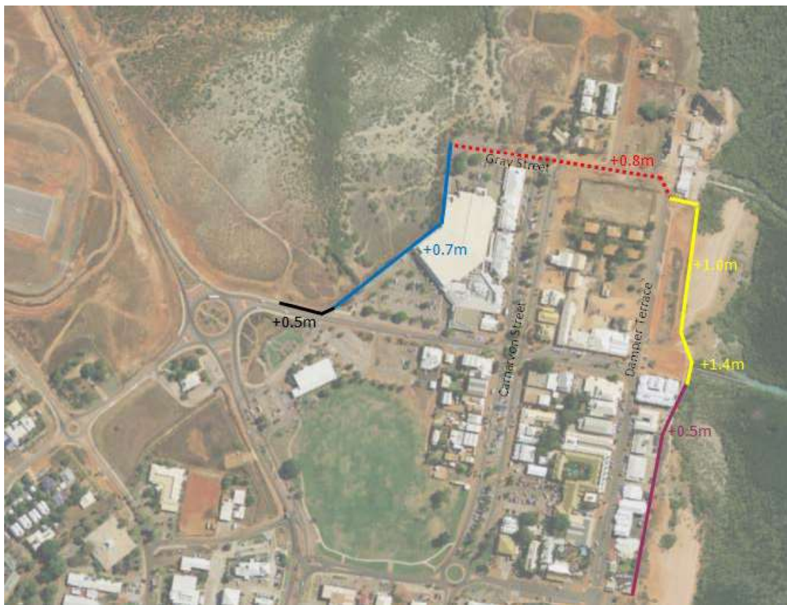
Figure 6.19: Chinatown Inundation Protection Option 1 – required height to raise current peninsula foreshore elements to meet 6.4m AHD.
