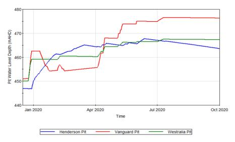
Figure 24: Modelled mine void water levels during active pumping.
