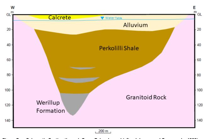
Figure 7 Schematic Section through Carey Paleochannel (after Johnson and Commander,1999)
