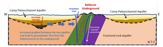
Figure 8 Schematic cross-section showing the aquifer relationship at Bellevue
