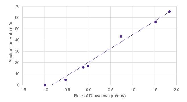
Figure 23 Observed rate of drawdown at various pump rates
