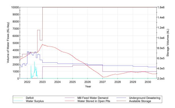
Figure 27: Scenario 2D — Water balance with high dewatering rate
