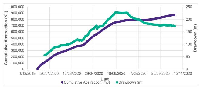
Figure 22: Cumulative volume abstracted and drawdown within the underground workings
