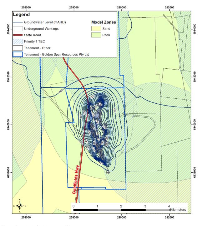
Figure 17 End of mining groundwater contours
