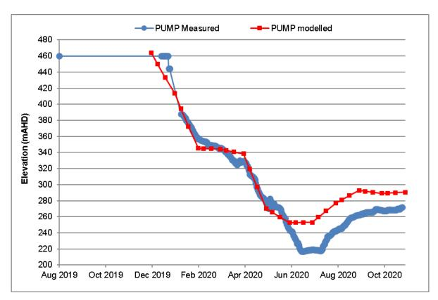
Figure 15 Measured vs modelled water level at pump location
