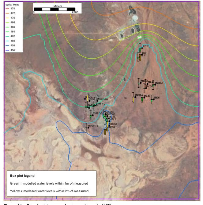
Figure 14 Steady state groundwater contours (mAHD)
