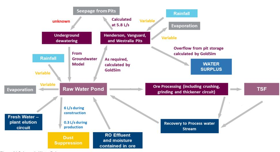
Figure 21 Schematic Water Balance
