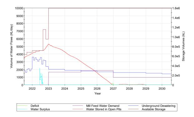
Figure 28: Scenario 3D — Water balance with averaged dewatering rate
