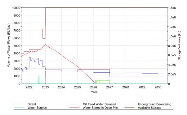
Figure 26 Scenario 1D — Water balance with low dewatering rate
