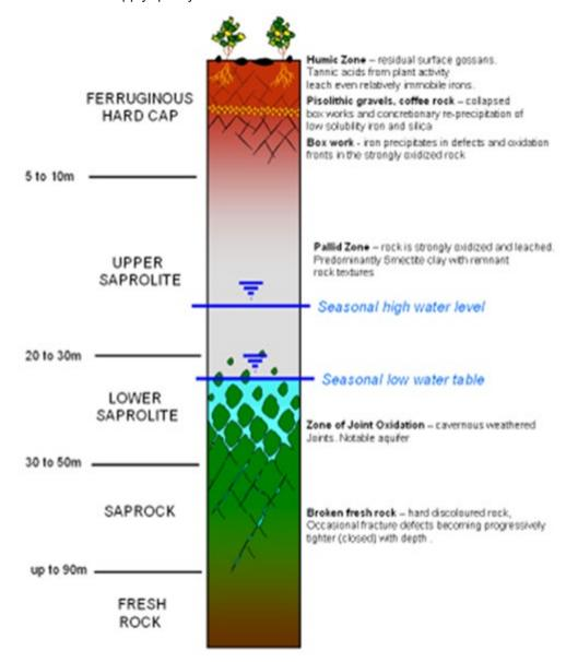
Figure 6 Schematic profile through a typical fractured-rock aquifer in the Goldfields
