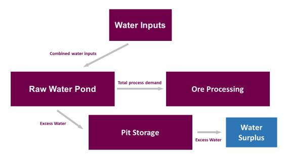
Figure 25 Simplified water balance flow diagram
