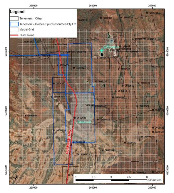
Figure 9 Model grid showing refinement over the Bellevue underground operations area
