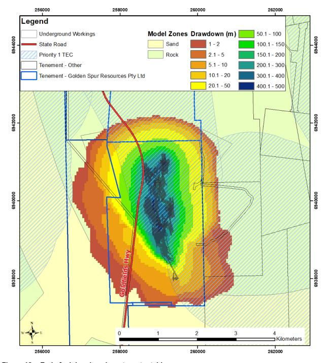
Figure 18 End of mining drawdown to water table
