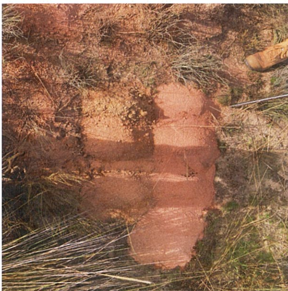
TP 5 150mm sand 300mm gravel Gravel clay to 2m Sandy/clay/white rock to 3m
