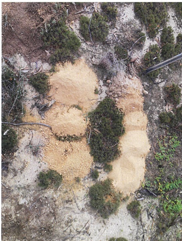
TP 5 150mm sand 300mm gravel Gravel clay to 2m Sandy/clay/white rock to 3m
