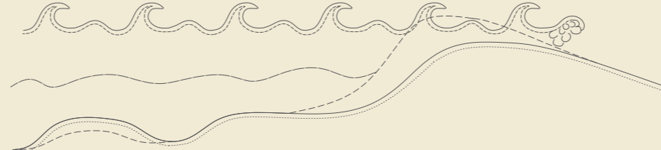
b DUNE OVERTOPPING
