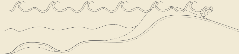
b DUNE OVERTOPPING
